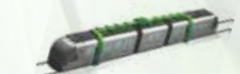
2. While it travels from one stop to another the Freedrive powers the traction system.
