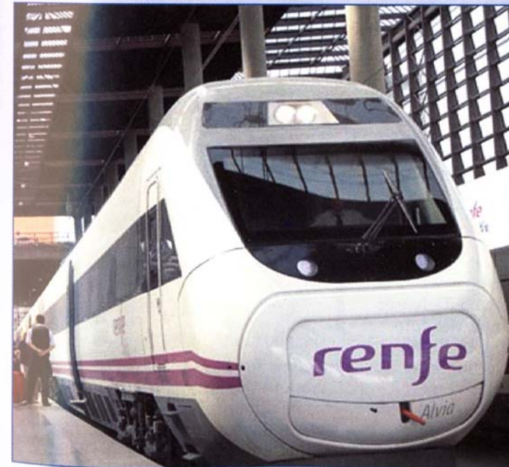
CAF's Brava gauge-changing equipment is fitted on the fleet of 12 Class 120 EMUs supplied to RENFE in conjunction with Alstom. Using the new gauge-changing installation at Roda de Barà, these will provide the fastest Madrid - Barcelona journey time of 4 h 15 min for the 612 km
