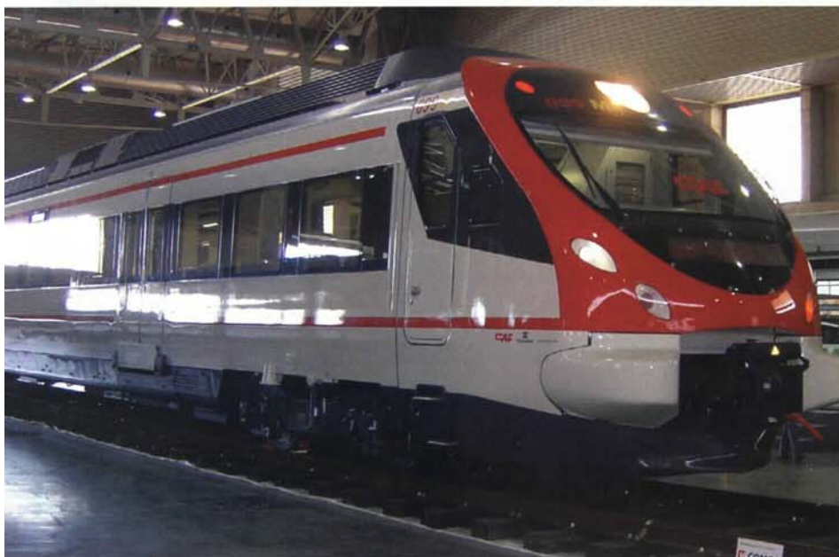
A Civia emu fitted with CAF traction equipment has run more than 25,000km under test.
