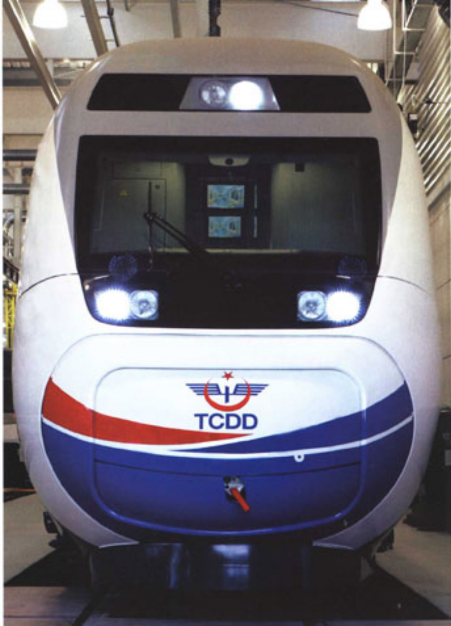
One of the new six-car 250km/h emus supplied by CAF to TCDD.
