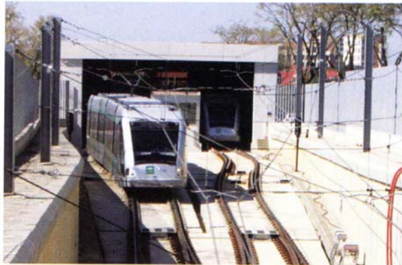
The line has a fleet of five-section 65 km/h CAF light rail vehicles, which are equipped for automatic train operation.
