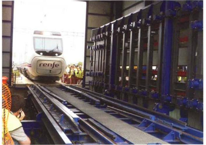
TCRS-1 uses vertically-mounted changers. With the Talgo platform folded away, the CAF platform is lowered into position (left), so that a CAF-built Series 120 EMU equipped with Brava variable-gauge wheelsets can pass through the changer at Roda de Barà (right).
