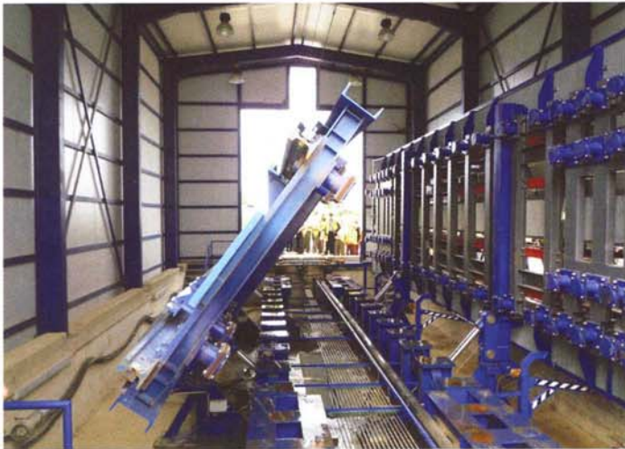
TCRS-1 uses vertically-mounted changers. With the Talgo platform folded away, the CAF platform is lowered into position (left), so that a CAF-built Series 120 EMU equipped with Brava variable-gauge wheelsets can pass through the changer at Roda de Barà (right).
