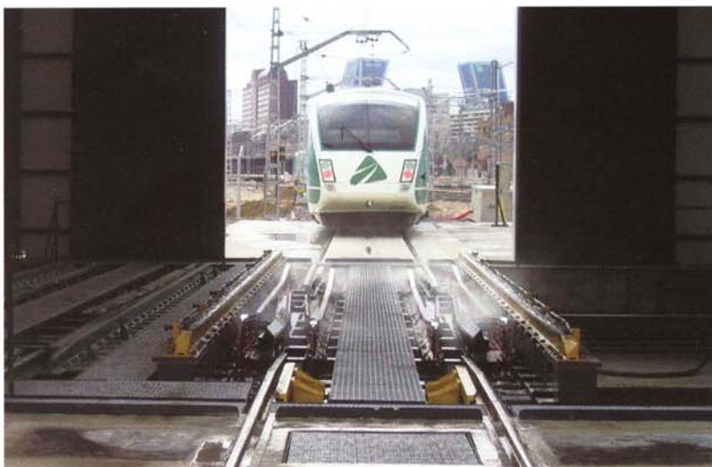
The TCRS-2 gauge-changers at Madrid Chamartín (above) and Valdestillas use horizontally-traversing platforms to speed the switch between systems.
