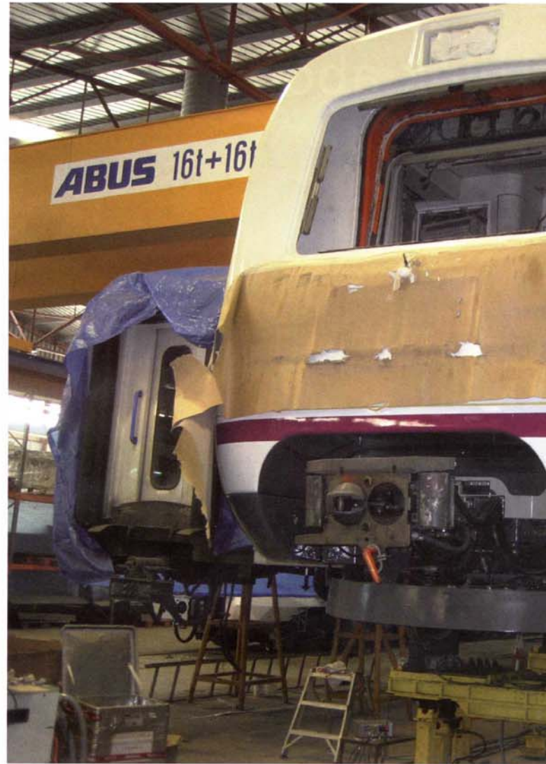
Fig. 5. Testing car on tilting platforms
